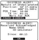
The **GX2200E** is capable of transmitting a DSC distress alert with the following "Nature of Distress" categories:
