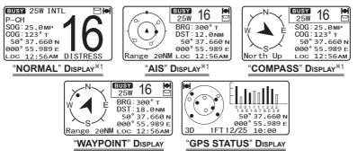
\*1: By default the COG in "NORMAL" and "COMPASS" displays and BRG in "AIS", "COMPASS". and "WAYPOINT" displays are set to "True", however this may be change to magnetic by following the steps in section "5.10 CHANGING COG TO TRUE OR MAGNETIC".
