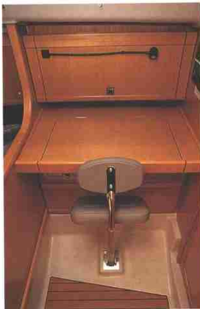
Above, the compact navigation station owes much of its comfort to the hingeing navigator's seat which provides security on either tack. Right, there is plenty of space around the saloon table set to starboard of the accommodation
