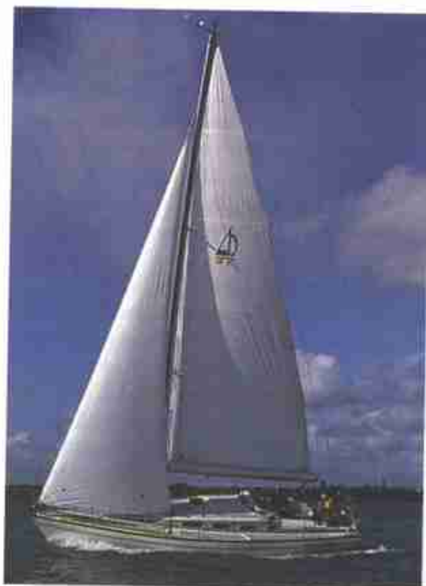
A fully battened mainsail and non-overlapping jib make for easy sail handling and good performance
