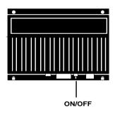
Set the ON/OFF switch of the main unit to the ON position. The system will automatically return to the same status as when it was switched OFF.
