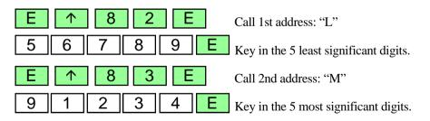
Before switching the unit OFF, check that the numbers are entered correctly:
