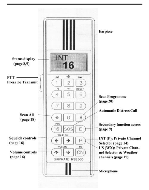
The **ON/OFF switch** is fitted at the base of the main unit and a stand-by facility on the handset allows power consumption to be reduced, so that the set can be left on almost indefinitely.
