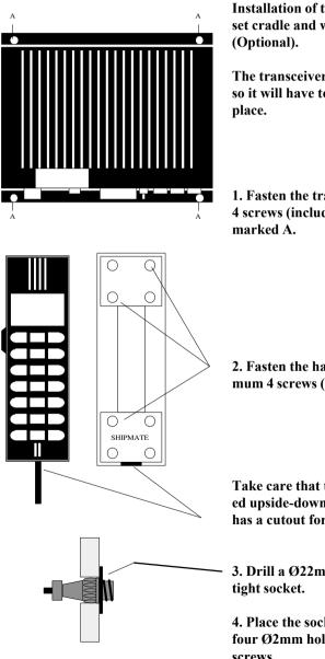
Installation of transceiver unit, handset cradle and watertight socket. (Optional).
